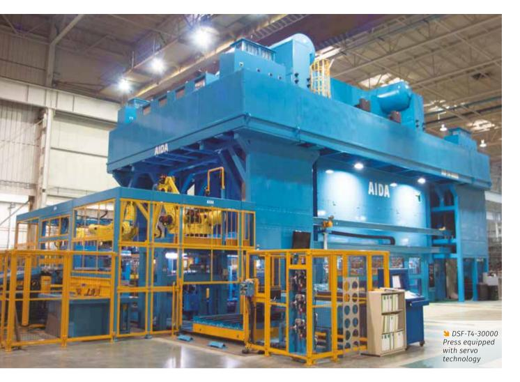
adjustments and test forming, and even high-difficulty shapes can now be efficiently and stably produced. Moreover, utilising a simulation program makes it possible to realise identical product quality in all the production facilities around the world that have the same types of servo presses.
